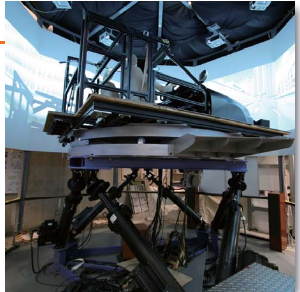
▲ Motion system with turntable mechanism
